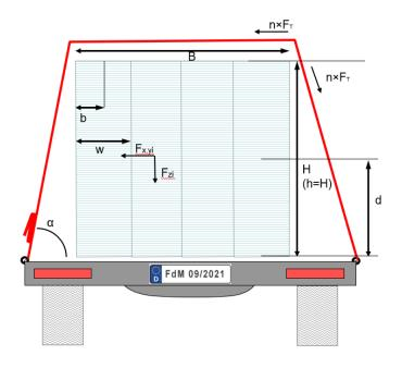
$$m \le \frac{2 \times 7 \times 350 \ daN \times (0.98 + 0.25 \times (4 - 1))s^2}{1.1 \times 9.81m \times (0.5 \times \frac{1.35m}{1.35m} \times 4 - 1)}$$
