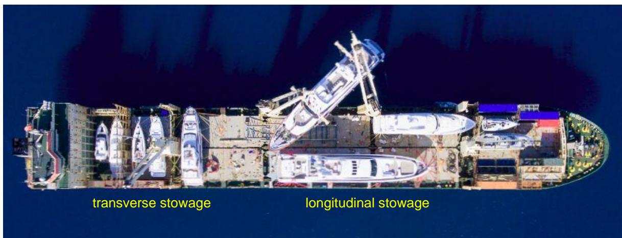
Figure 1: Cargo stowed in longitudinal and transverse orientation
